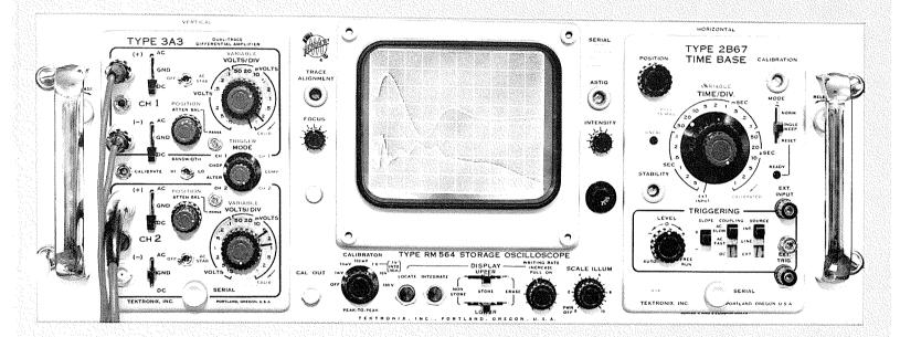
UP TO 500 CM/MSEC SINGLE-SHOT WRITING SPEED REMOTE CONTROLLED DISPLAY ERASE OVER ONE HOUR VIEWING TIME OF SINGLE-SHOT SIGNALS SELECTABLE HORIZONTAL AND VERTICAL AXIS PLUG-INS X-Y DISPLAYS
