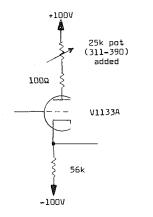
Figure 5. Partial schematic showing the addition of the 25 k potentiometer to the plate circuit of V1133A.
