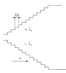
Figure 3. Output of twelve-turn transformer.
