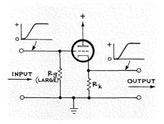
Fig. 5 — Illustrating that the polarity of the cathode-follower output-signal voltage is the same as that of the input-signal voltage — in contrast to the polarity reversal that occurs in the plate-loaded amplifier.
