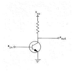
Figure 4 — Amplifier used as an example of the application of transresistance compared to h-parameters. The DC operating point is assumed to be set at  $l_c = 5 \text{ ma}$ ;  $V_{cc} = 2.5 \text{ v}$ . The transistor is a 2N2475.
