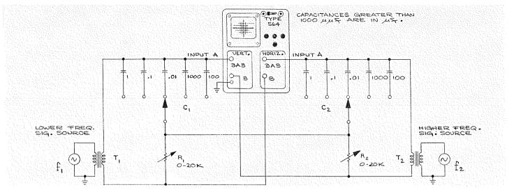
Fig. 1. Circuitry For Displaying Roulette Patterns.
