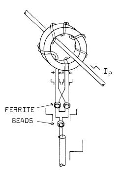
Figure 5. Twelve-turn bifilar winding.
