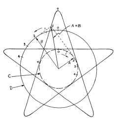
Fig. 5. Graphical construction of a roulette pattern for a frequency ratio of 3:2.
