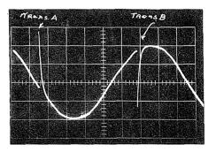
Figure 1. Power-line waveform with simulated transients.
