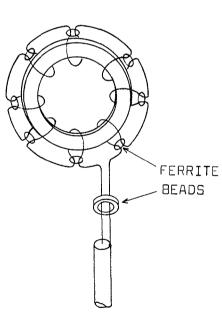
Figure 7. Eight-turn multifilar winding.
