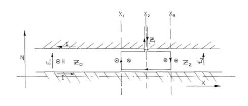
Figure 1. A single-turn winding inserted in the space between the inner and outer conductor of a coaxial transmission line of impedance  $Z_{\rm o}$ .
