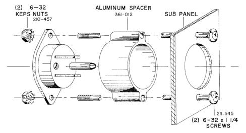
Fig. 3. Pictured instructions for recessing the 3-wire connector on instruments using a detachable, 3-conductor power cord.
