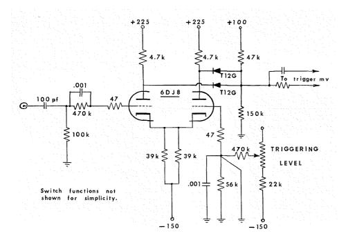
Figure 2. Modified Trigger-Amplifier Circuit of a Type 530 or Type 540 Series Oscilloscope.
