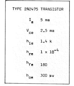
Table 1 — List of the h-parameters for the Type 2N2475 transistor at  $I_e\equiv$  5 ma;  $V_{ce}\equiv$  2.5 v.
