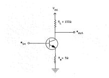
Figure 5 — Amplifier with the same type transistor set at the same operating point as that in Figure 4. This circuit has  $R_{\circ}$  added to reduce the voltage gain and increase the input resistance.
