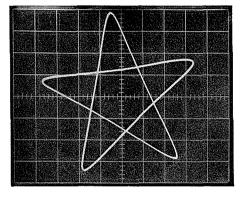
Fig. 6. Roulette pattern for a 3:2 frequency ratio.
