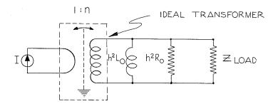
Figure 8. Lumped-constant equivalent circuit of a current transformer.
