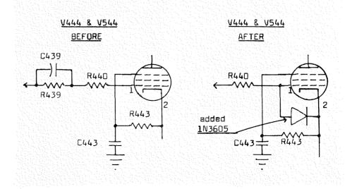
Figure 4. "Before" and "After" schematic for replacing the 0.01 µf/47 k RC network, in the grid circuit of both V444 and V544, with 1N3605 diodes.
