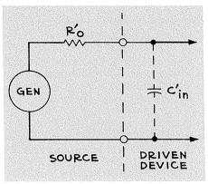
Fig. 3 — Here a second signal source whose internal impedance is  $R'_{\circ}$  drives a circuit whose input capacitance is  $C'_{in}$ . One way to keep the time constant  $R'_{\circ}C'_{in}$  short is to make  $R'_{\circ}$  very small. Then the risetime is short even if  $C'_{in}$  is relatively large.
