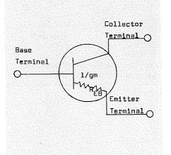
Figure 2 — Schematic equivalent of the emitter circuit of a transistor. 1/gm is the dynamic resistance of the junction due to carrier action and  $R_{EB}$  is the DC resistance in the leads and ohmic contacts of the leads within the transistor case.
