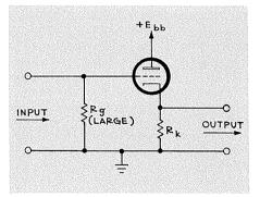
Fig. 1 — Basic cathode-follower circuit. Here the load resistor  $R_k$  is connected in the cathode circuit, rather than in the plate circuit as in the plate-loaded amplifier.
