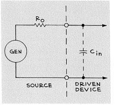
Fig. 2 — Here a signal source has an internal impedance  $R_o$ . The source drives a circuit whose input capacitance is  $C_{in}$ . If the time constant  $R_oC_{in}$  of this arrangement is small, then the risetime of the combination is short. One way to keep the time constant small is to make  $C_{in}$  very small. Then the risetime is short even if  $R_o$  is relatively large.
