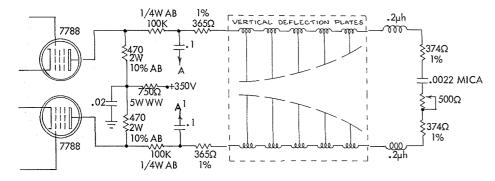
Figure 2. Type 580 Series Oscilloscope — Vertical-output circuit for direct connection to crt vertical plates.
