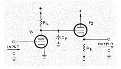
Fig. 11 — Here a plate-loaded amplifier V<sub>1</sub> drives the input of a cathode follower V<sub>2</sub>. The plate-to-ground capacitance of V<sub>1</sub> (plus the small input capacitance of V<sub>2</sub>) is represented by C<sub>p</sub>. The risetime of the coupling circuit between V<sub>1</sub> and V<sub>2</sub> is determined by the time constant R<sub>L</sub> C<sub>p</sub>.
